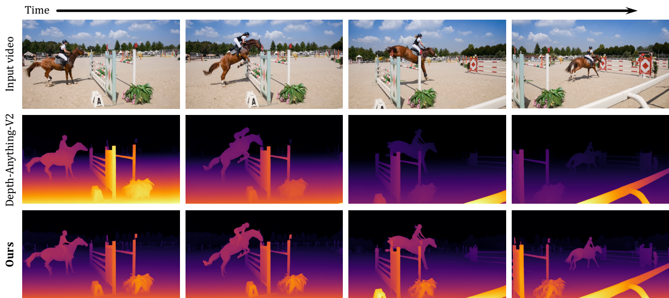
Figure 1. We innovate DepthCrafter, a novel video depth estimation approach, by leveraging video diffusion models. It can generate temporally consistent long depth sequences with fine-grained details for open-world videos, without requiring additional information such as camera poses or optical flow.
