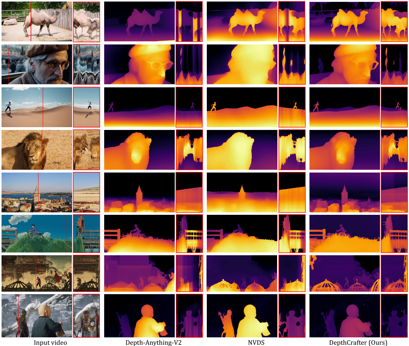
Figure 4. Qualitative comparison for open-world video depth estimation. We compare with the representative single-image depth estimation method Depth-Anything-V2 [68] and the video depth estimation method NVDS [63]. For better visualizing the temporal quality, we show the temporal profiles of each result in red boxes, by slicing the depth values along the time axis at the red line positions.
